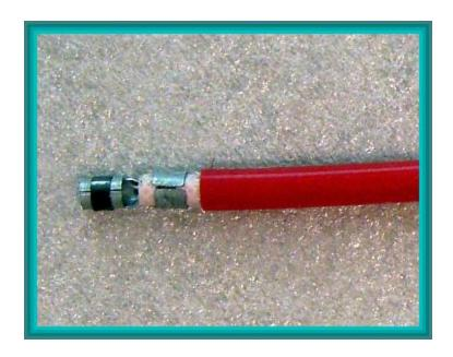
Insert the wire into the terminal with the core next to the bottom of the terminal and form the terminal tabs around the wire to hold it in place for crimping. Now crimp the terminal around white insulation.
